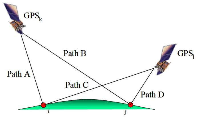
DD = (Path A - Path B) - (Path C - Path D)
